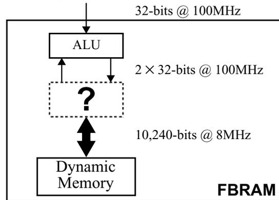
Figure 1. Bandwidth mismatch between pixel ALU and DRAM.
