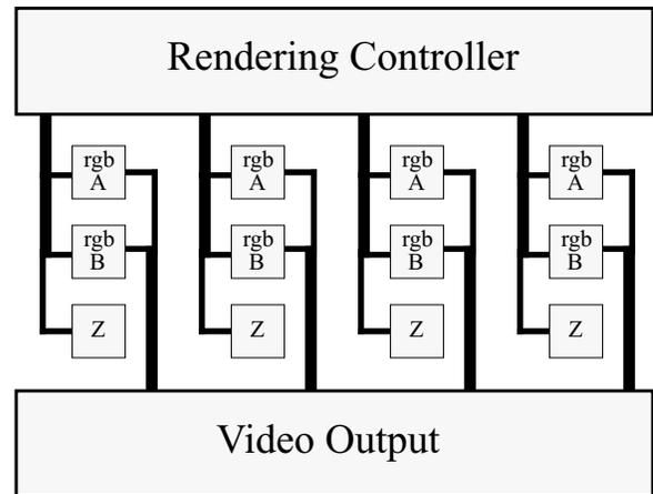
Figure 3. A four-way interleaved frame buffer system composed of 12 FBRAMs (1280x1024, double buffered 32-bit RGBα plus 32-bit Z).
