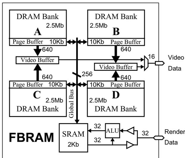
Figure 2. Internal block diagram of a single FBRAM.
